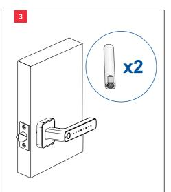
Screw the two (2) posts (groove side) onto the small black screws attached to the inside face of the outside lever. Place the outside lever onto the door ensuring posts go through latch.
