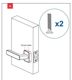
Place the inside lever onto the door. Line up holes with posts, then using the two (2) screws provided, secure the inside and outside levers onto the door. Note: Do not overtighten the screws.
