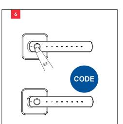
With door open try to unlock the lock and make sure the installation was successful. In factory default mode, the lock will unlock with any code or any finger print.
